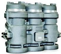
The Woodward VariStroke solves the #1 turbine reliability problem: dirty oil. Designed to operate on dirty turbine lube oil with no special filters needed, the VariStroke has one moving servo part, a self-cleaning rotary control valve and corrosion-resistant components. This integrated actuator is intended for use on mechanical-drive or generator drive steam turbines, and uses a low-pressure hydraulic oil source (typically turbine lube oil) to provide its output shaft force.
