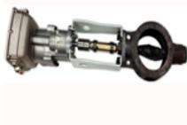
Woodward's Glo-Tech hot valve system provides precise control of high temperature gases in an on-engine environment. The Glo-Tech hot valve system is a high-temperature butterfly valve and electric actuator combination that can be used to regulate high-temperature gases in single and two-stage turbocharged reciprocating engines. The valve is designed to be positioned by an R-Series electric rotary actuator through an anti-backlash coupling capable of handling considerable misalignment.
