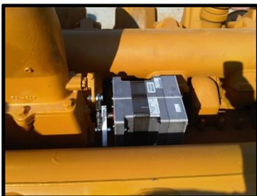
All versions of the E<sup>3</sup> control system offer an important feature that differentiates it from the competition. The system includes an integrated digital speed controller that can replace an existing mechanical governor or older analog electronic speed control. This option allows the speed control to be integrated with the air/fuel ratio control in the same unit which improves emissions control and engine stability since these two fundamental functions are designed to work together.
